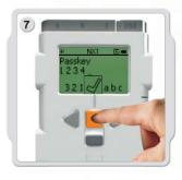
If you connect to a device for the first time, your NXT asks for a Passkey. Just press Enter to use the default passkey 1234 or make up your own code. The other Bluetooth device must know your passkey in order to confirm the connection. This means the two NXT bricks need to enter the same passkey in order to connect.
