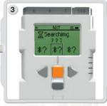
Depending on how many are detected in the area, the Bluetooth devices will appear in a list on the NXT display after a few seconds.
